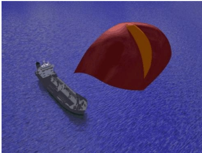
Figure 8. KiteShip Concept Applied To Commercial Cargo Ship
