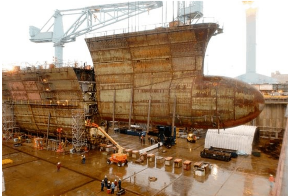
Figure 1. Bulbous Bow Section For CVN-77
