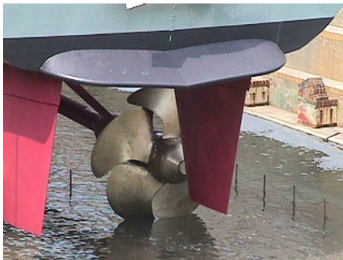
Figure 3. Stern Flap On DDG-51 Class Destroyer
